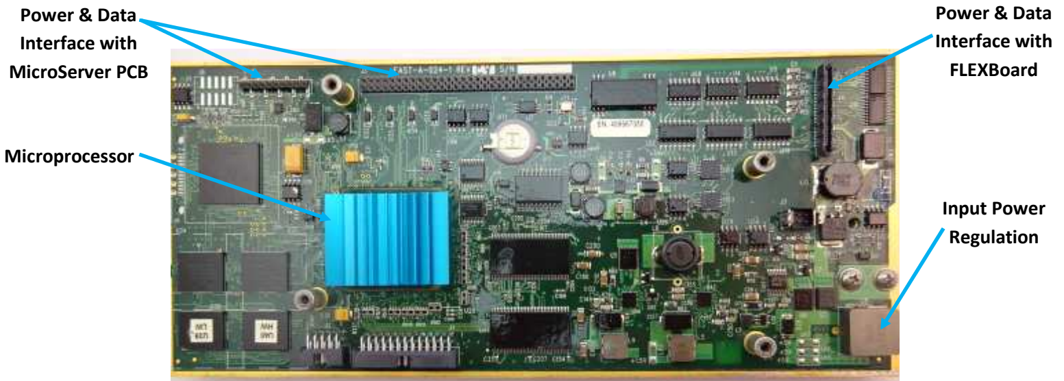
Figure 3: Control Processor Top View
