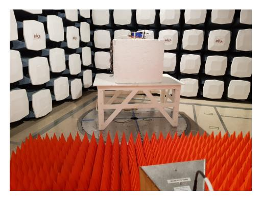
7.4 Radiated Emission above 1 GHz Rear View
