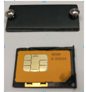
Figure 5: SIM Card Door & Tray
