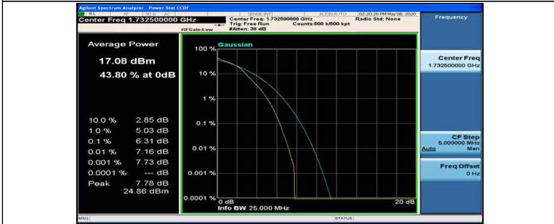
(Channel Bandwidth: 5 MHz)_MCH_16QAM_12RB#13
