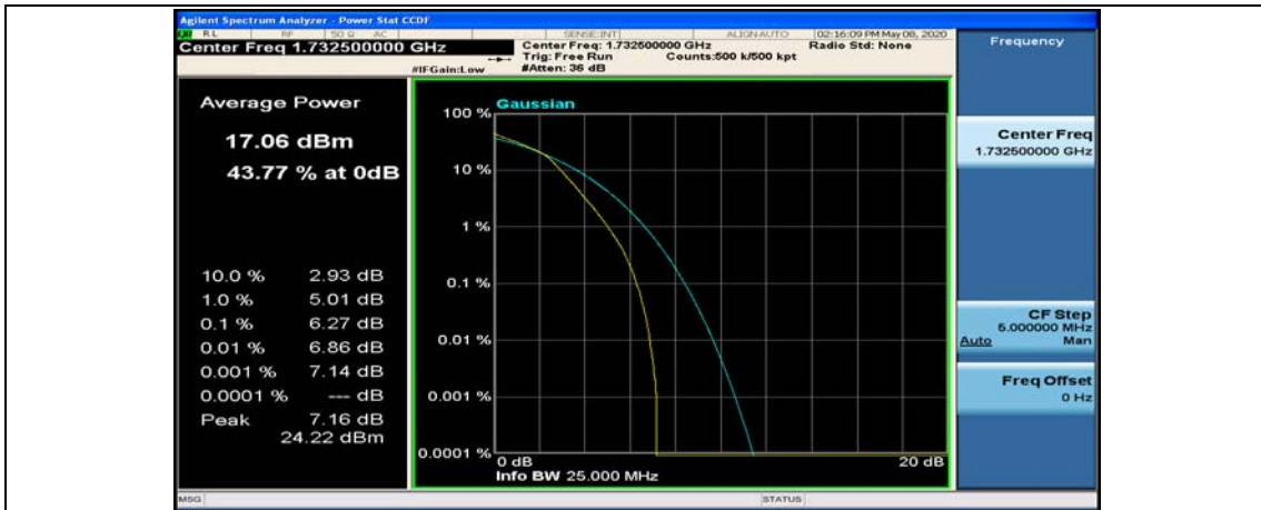
(Channel Bandwidth: 3 MHz)_MCH_16QAM_15RB#0
