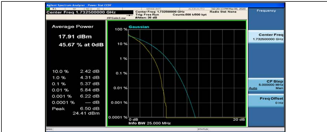
(Channel Bandwidth: 5 MHz)_MCH_QPSK_25RB#0
