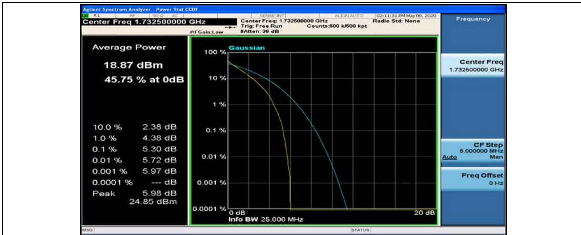
(Channel Bandwidth: 1.4 MHz)_MCH_QPSK_6RB#0
