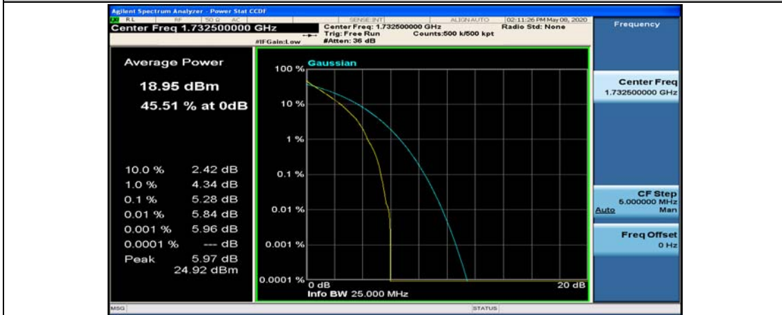
(Channel Bandwidth: 1.4 MHz)_MCH_QPSK_3RB#3
