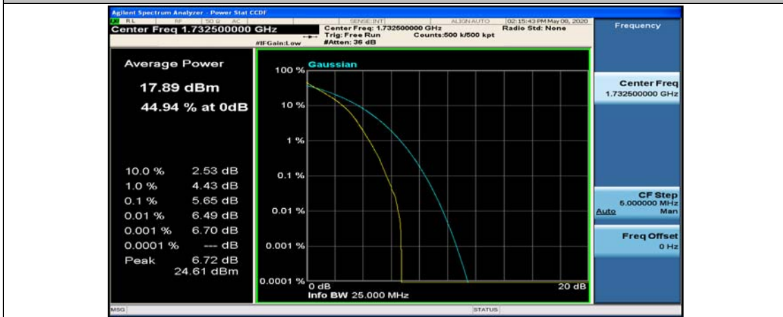
(Channel Bandwidth: 3 MHz)_MCH_QPSK_8RB#4
