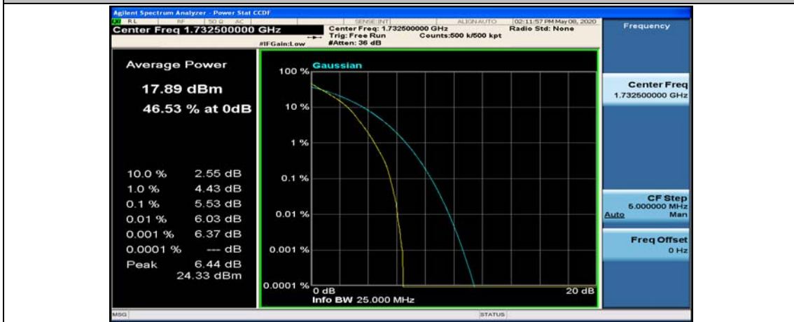
(Channel Bandwidth: 1.4 MHz)_MCH_QPSK_6RB#0
