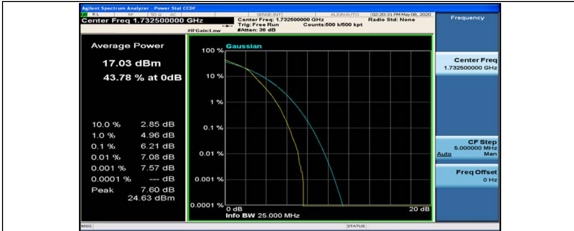
(Channel Bandwidth: 5 MHz)_MCH_16QAM_25RB#0
