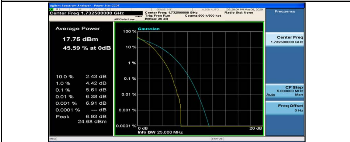
(Channel Bandwidth: 5 MHz)_MCH_QPSK_12RB#6
