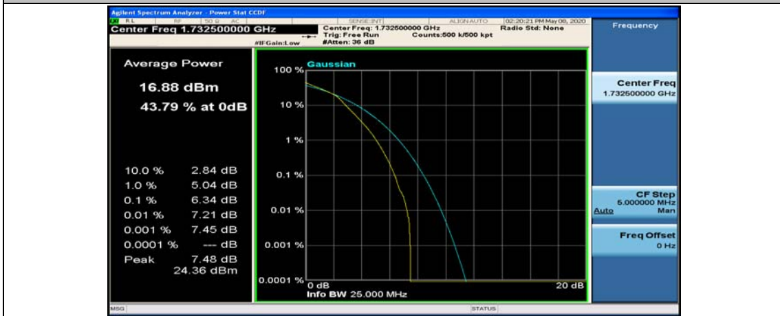
(Channel Bandwidth: 5 MHz)_MCH_16QAM_12RB#6
