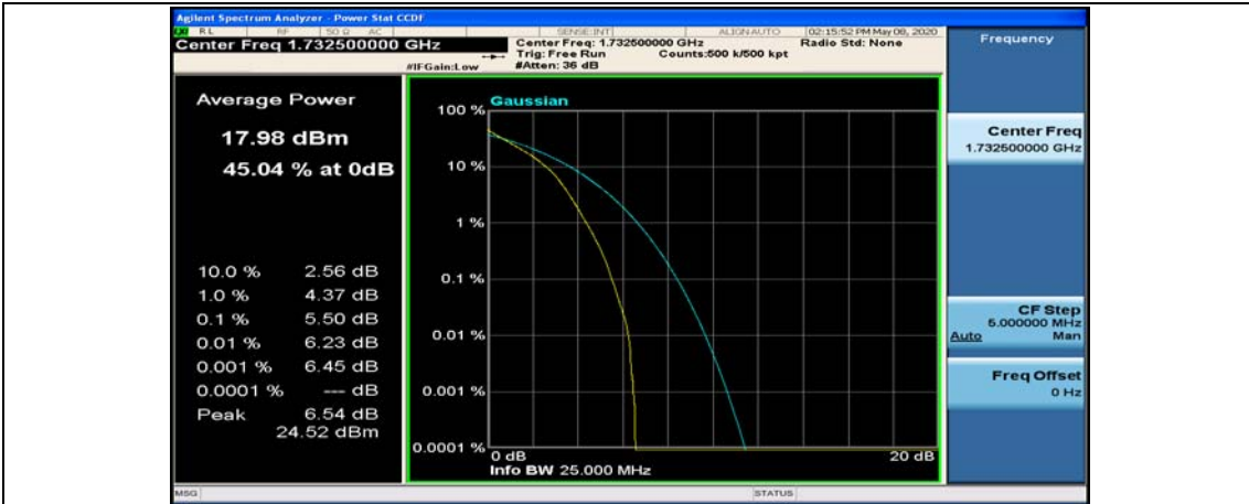
(Channel Bandwidth: 3 MHz)_MCH_QPSK_15RB#0
