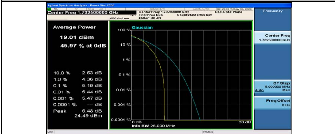
(Channel Bandwidth: 5 MHz)_MCH_QPSK_1RB#24
