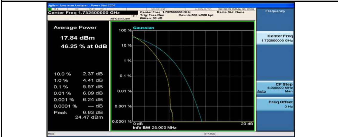
(Channel Bandwidth: 5 MHz)_MCH_QPSK_25RB#0
