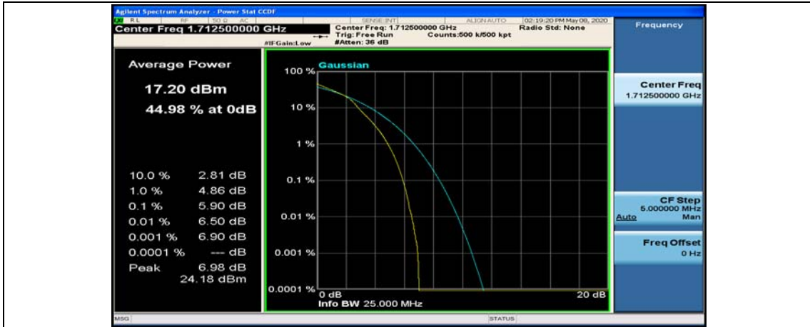
(Channel Bandwidth: 5 MHz)_MCH_16QAM_1RB#0
