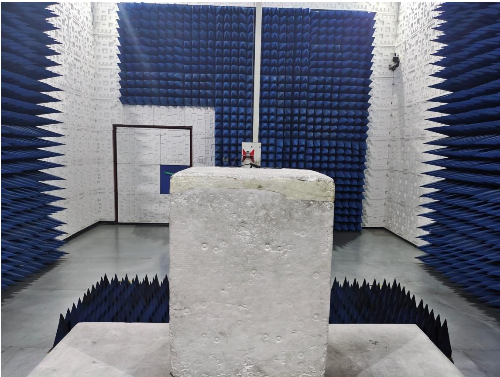
RADIATED EMISSION TEST SETUP ABOVE 1GHZ
