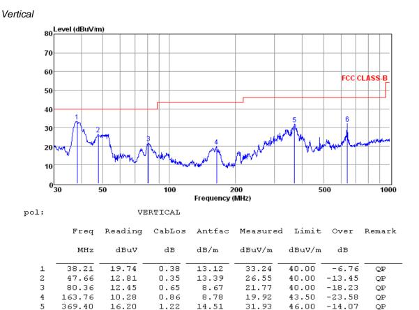
2. Measured= Reading + Antenna Factor + Cable Loss
