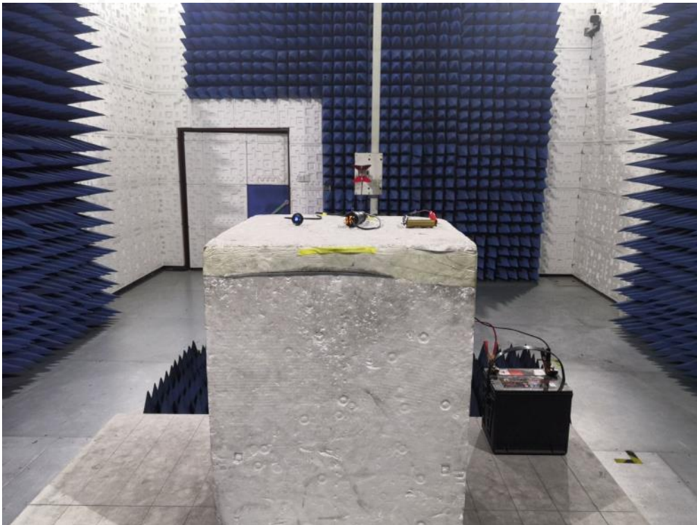
RADIATED EMISSION TEST SETUP ABOVE 1GHZ
