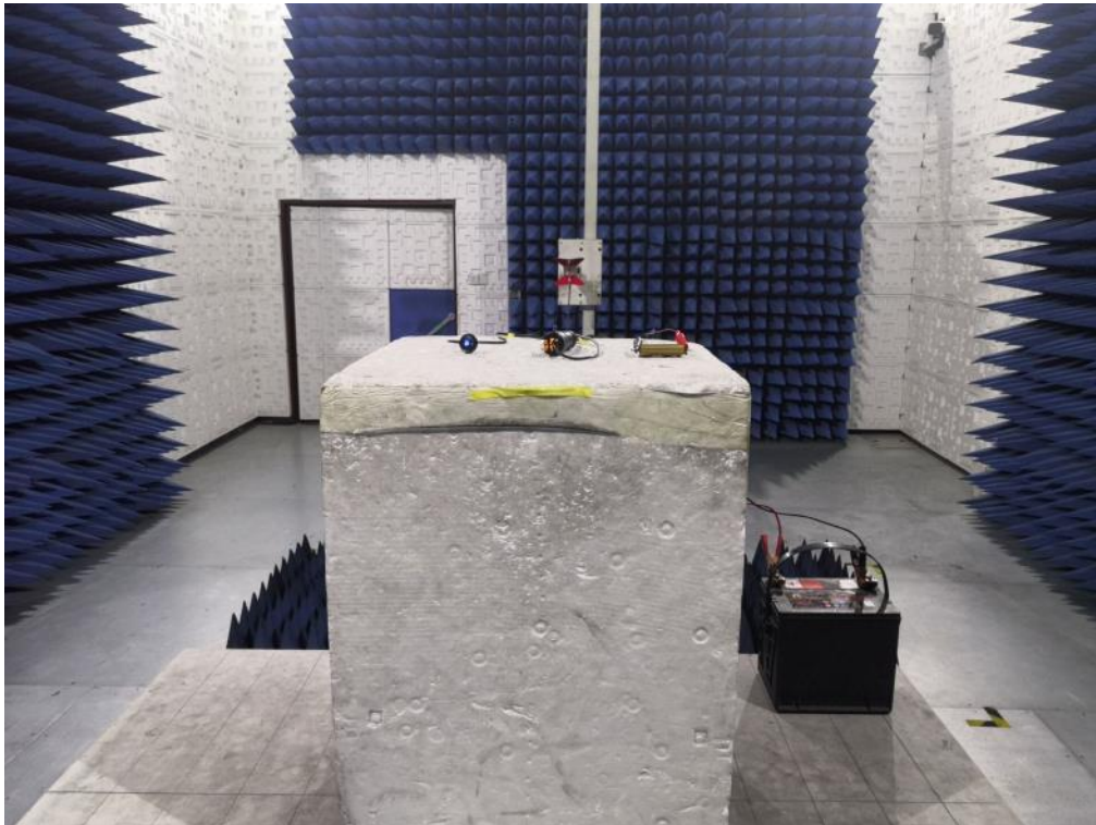
RADIATED EMISSION TEST SETUP ABOVE 1GHz
