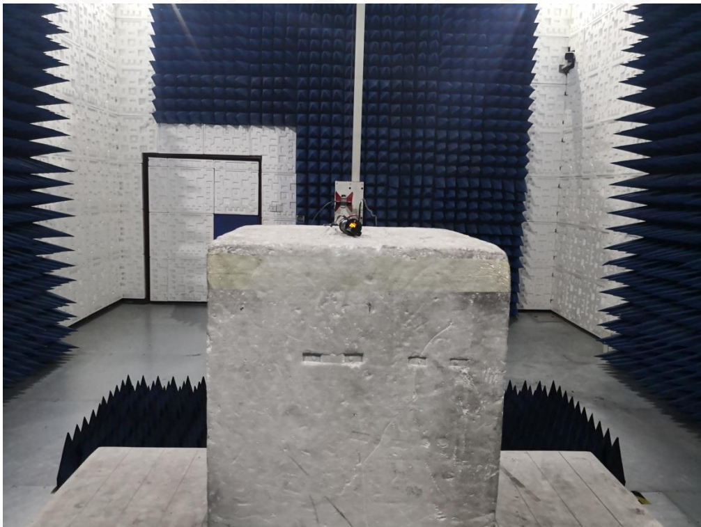
RADIATED EMISSION TEST SETUP ABOVE 1G
