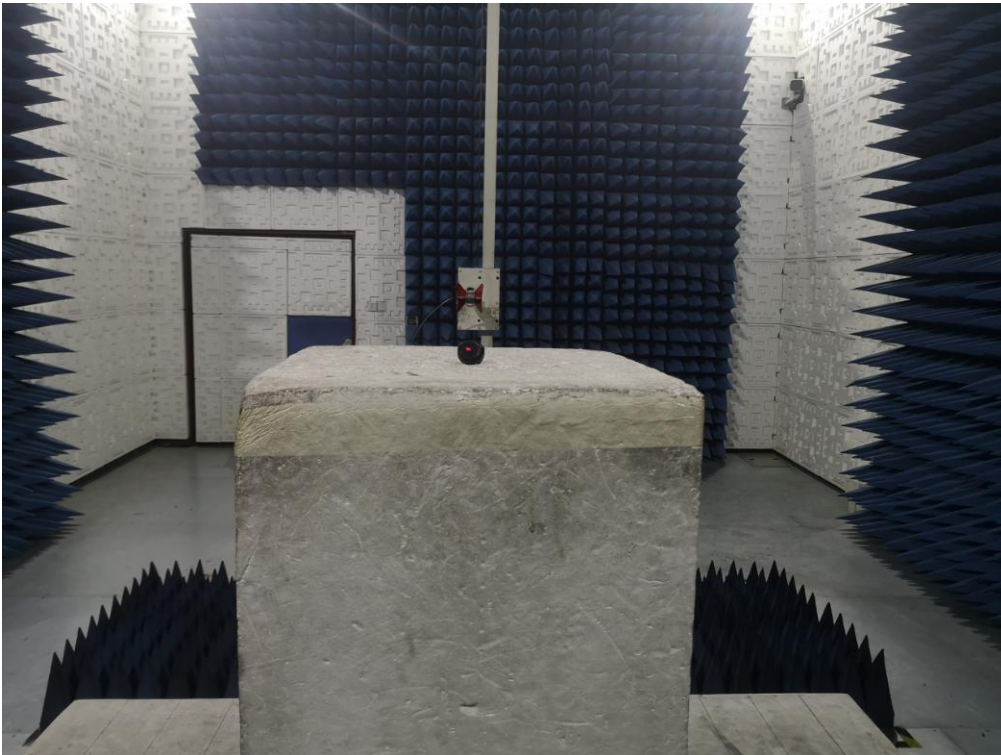
RADIATED EMISSION TEST SETUP ABOVE 1GHz
