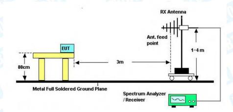
Below 1000MHz Test Setup
