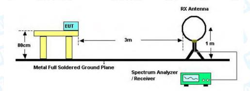
Below 30MHz Test Setup
