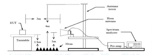
Above 1GHz Test Setup
