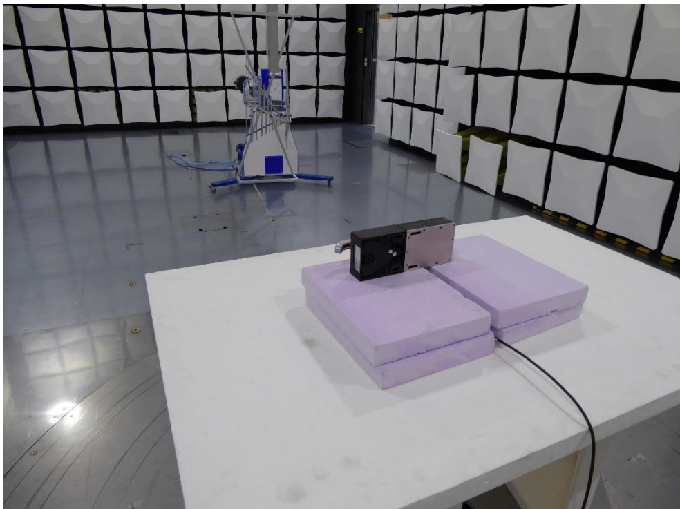
Test setup semi anechoic chamber (30 MHz to 1 GHz)
