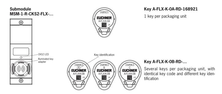
The submodule MSM-1-R-CKS2-FLX-... has a key adapter with integrated evaluation electronics. The submodule forms a safe system together with a corresponding key and forwarding of the evaluated data to the bus module MBM. The key determines the function. You will find further information in chapter 10.1. Configuring the key adapter and teaching-in the key for the first time on page 8.
