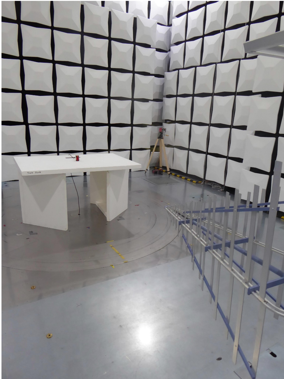
Test setup semi anechoic chamber M276; Preliminary and final measurement 30 MHz – 1 GHz
