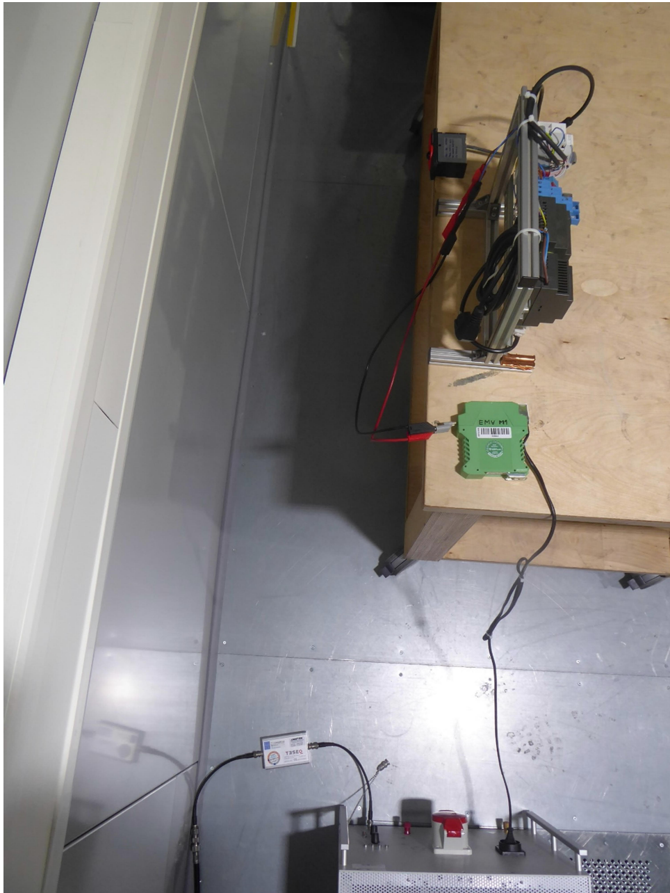
Test setup shielded room M155; Conducted emissions
