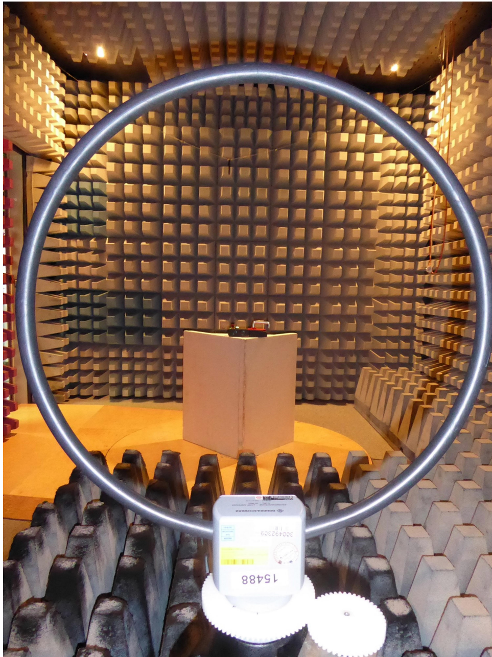
Test setup anechoic chamber M20; Preliminary measurement 9 kHz to 30 MHz
