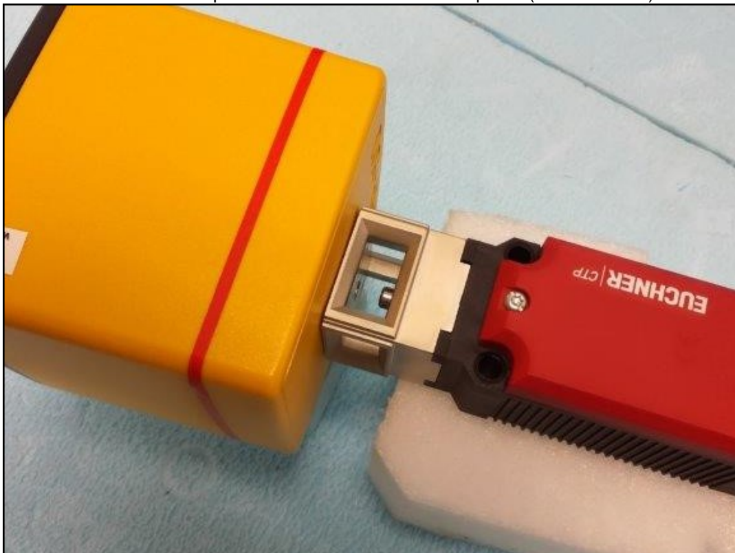
Photo 14: Test position - DUT A with EHP-50 F probe (0mm distance)
