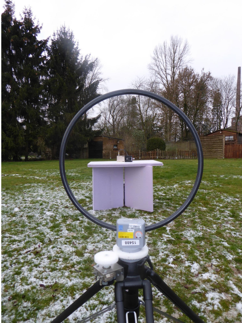
182138_Set9.JPG: Test setup open area test site, 9 kHz – 30 MHz @ 3m
