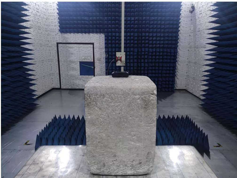
RADIATED EMISSION TEST SETUP ABOVE 1GHz
