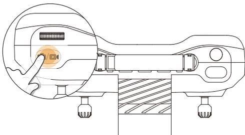
**Take Photo:** Short press the
