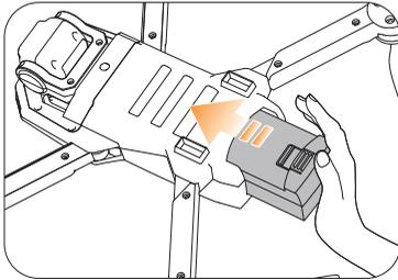
Push the battery correctly into the drone. Make sure that you hear a click sound, which indicates that the battery is firmly installed.
