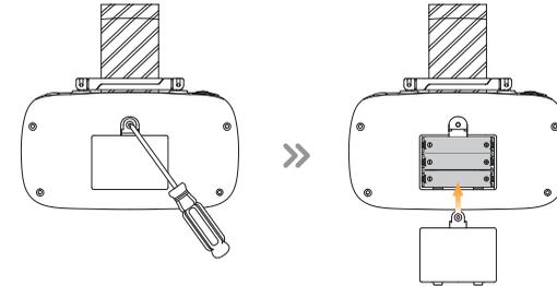
Open the battery cover on the back of the transmitter. Put in three AAA batteries (not included). Then, close the cover.
