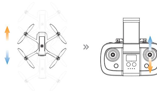
**3 Deactivate Trim Mode:** Once adjustments are made, long press the Trim button or stop operating the joysticks for 2 seconds to exit Trim Mode.
