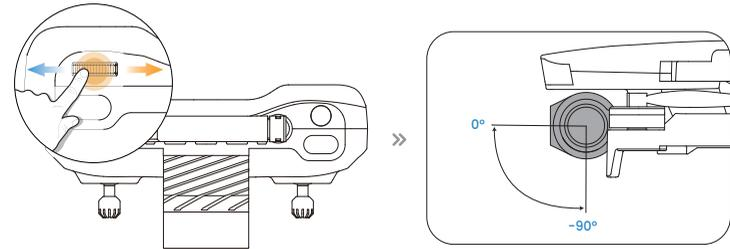
Adjust the camera angle by scrolling the camera adjustment dial
