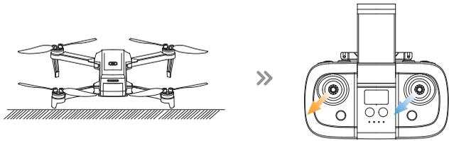
Make sure to place the drone on a level surface before calibrating the gyro. Simultaneously push the left joystick and the right joystick to the bottom left corner to calibrate the gyro. The indicator lights on the drone will blink, then turn solid, which indicates that the calibration is completed.
