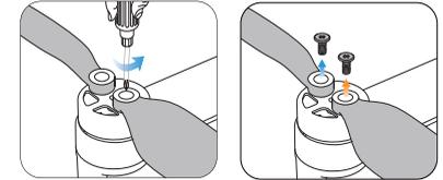
For propeller removal, use a screwdriver (provided) to rotate the screws counter-clockwise and remove the propellers. Be sure to hold the motor while detaching the propeller.
