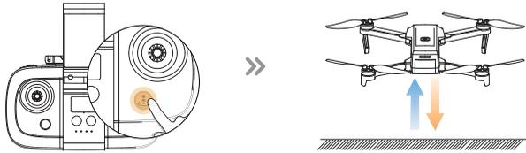
**Takeoff** Short press the
