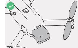
Make sure the drone battery and the propellers are mounted securely.
