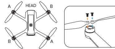
The drone will not fly unless the correct propeller is installed on the correct motor shaft. Each propeller is labeled with either an "A" or "B" on it. Secure the propeller onto the motor shaft using screws, turning each screw clockwise.
