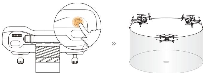
Long press the
