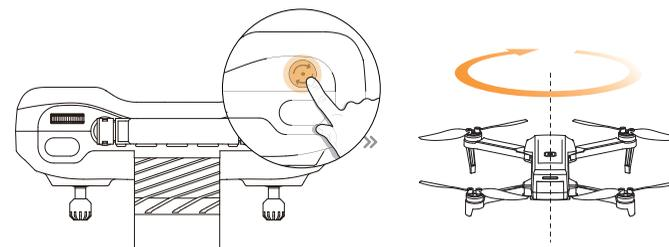
Short press the
