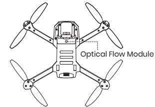
The Optical Flow Positioning System consists of a camera module, which acquires the position information of the drone through visual images to ensure precise positioning of the drone. The optimal usage height for Optical Flow Mode is 1.6-9.8ft.
