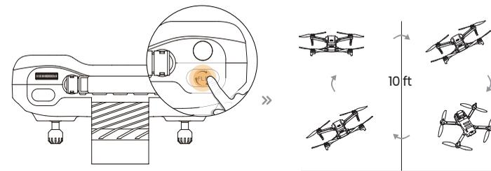
After you get familiar with all the functions of the drone, you can try this amazing flip mode. When the drone is at least 10 ft from the ground, press down on the
