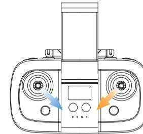
Simultaneously push the left joystick to the bottom right corner and the right joystick to the bottom left corner. The motors will rotate, and the drone is unlocked.
