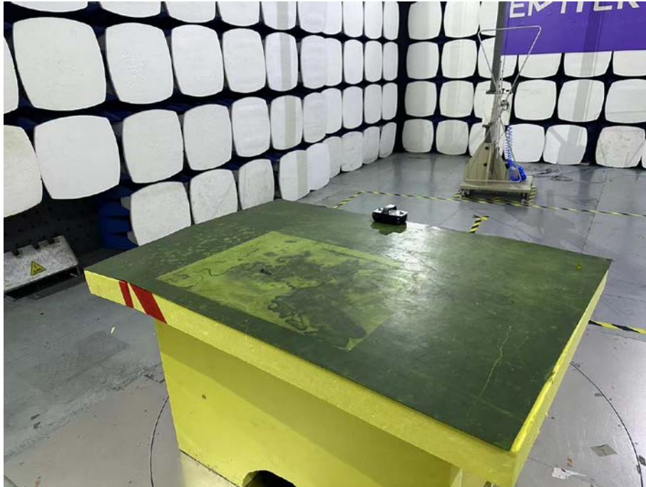
Spurious Emission Test Setup (Below 1GHz)
