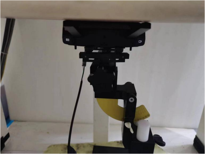
Fig-4.2 Open the Rear Face antenna lengthwise of EUT with 0 cm Gap (Body Mode)
