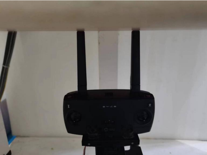
Fig-4.3 Open the Top Side antenna lengthwise of EUT with 0 cm Gap (Body Mode)
