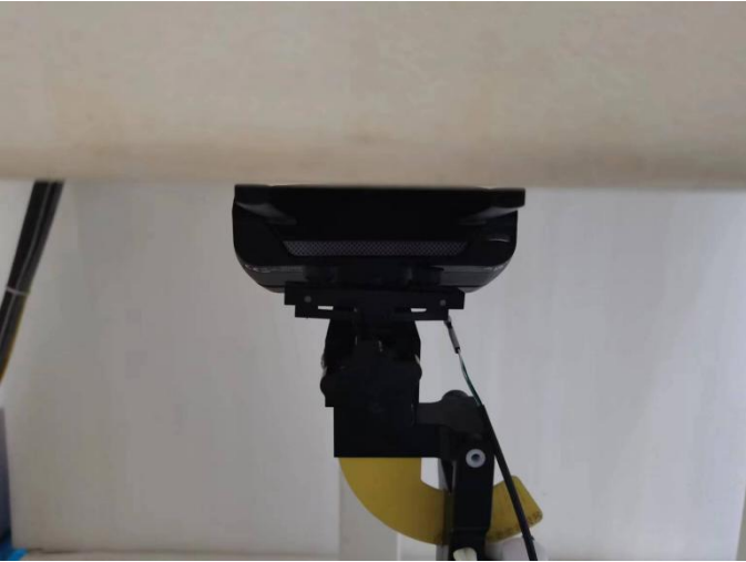
Fig-4.1 Open the Front antenna lengthwise of EUT with 0 cm Gap (Body Mode)
