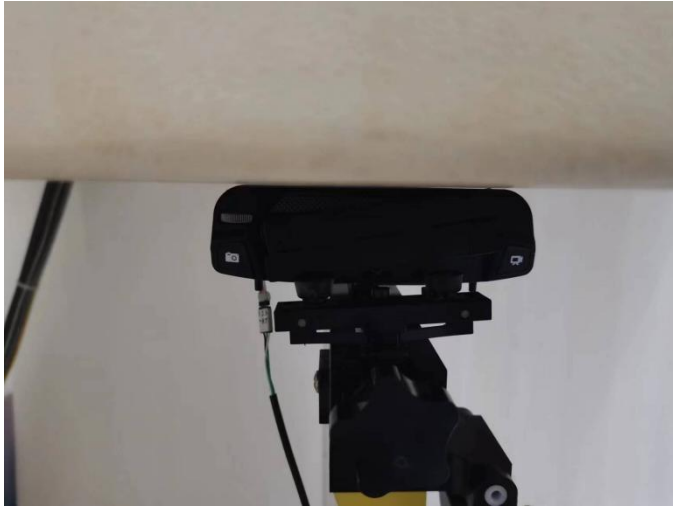
Fig-4.9 Close the Rear Face antenna of EUT with 0 cm Gap (Body Mode)
