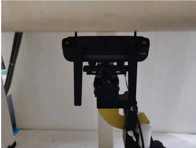
Fig-4.5 Open the Front antenna lateral of EUT with 0 cm Gap (Body Mode)
