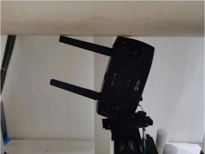
Fig-4.4 Open the Right Side antenna lengthwise of EUT with 0 cm Gap (Body Mode)
