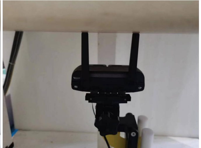
Fig-4.6 Open the Rear Face antenna lateral of EUT with 0 cm Gap (Body Mode)
