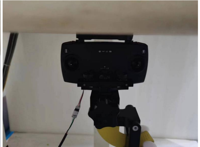
Fig-4.10 Close the top antenna of EUT with 0 cm Gap (Body Mode)
