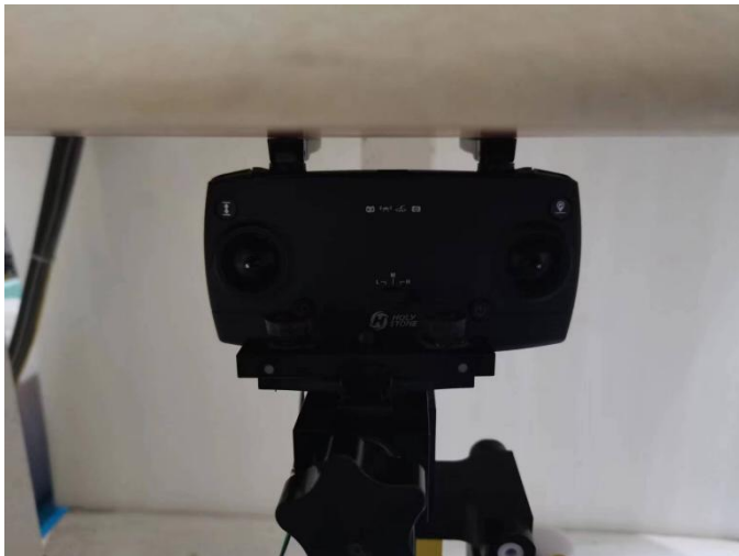
Fig-4.7 Open the Top antenna lateral of EUT with 0 cm Gap (Body Mode)
