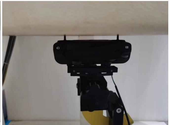
Fig-4.8 Close the Front antenna of EUT with 0 cm Gap (Body Mode)
