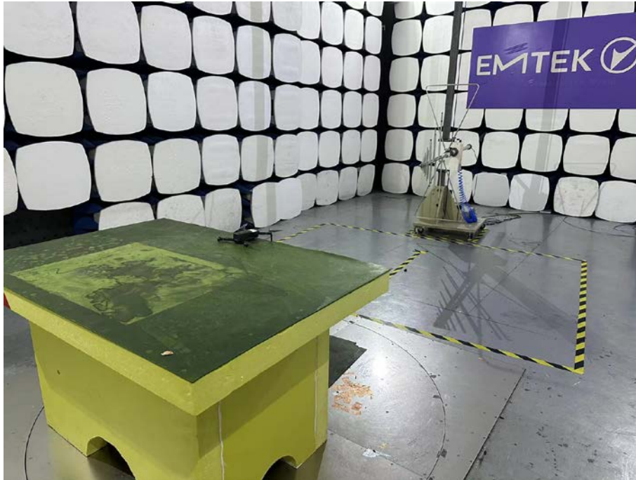
Spurious Emission Test Setup (Below 1GHz)
