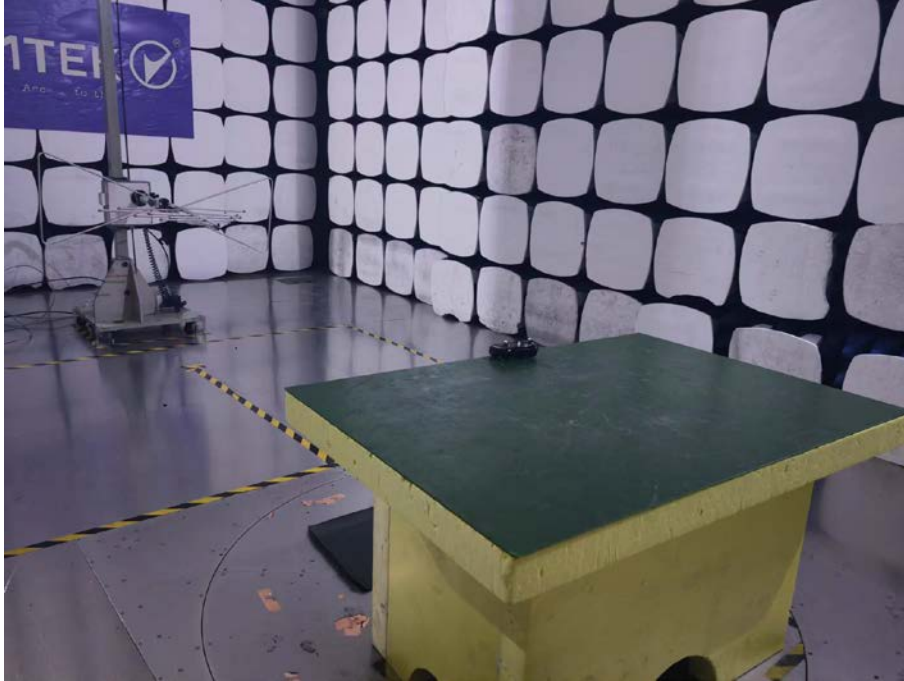
Spurious Emission Test Setup (Above 1GHz)
