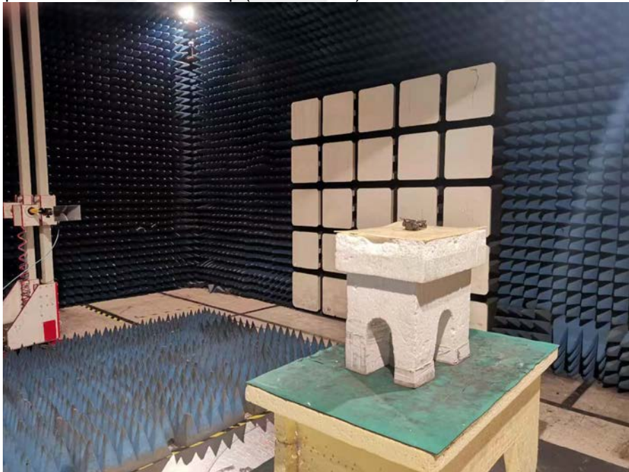
Spurious Emission Test Setup (Above 1GHz)
