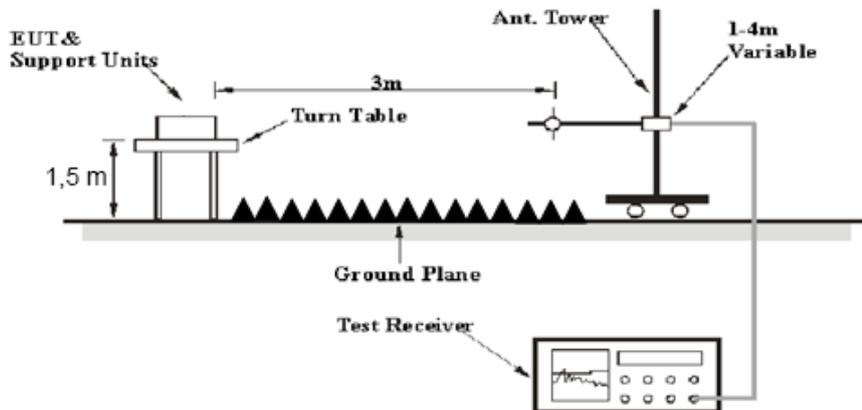
The radiated emission Below 1GHz tests were performed in the 3 meters chamber test site A, above 1GHz tests were performed in the 3 meters chamber test site B, using the setup accordance with the ANSI C63.10-2013. The specification used was the FCC 15.209, and FCC 15.247 limits.
