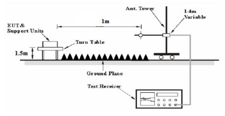
The radiated emission tests were performed in the 3 meters chamber test site, using the setup accordance with the ANSI C63.10-2013. The specification used was the FCC 15.209, FCC 15.249 limits.
