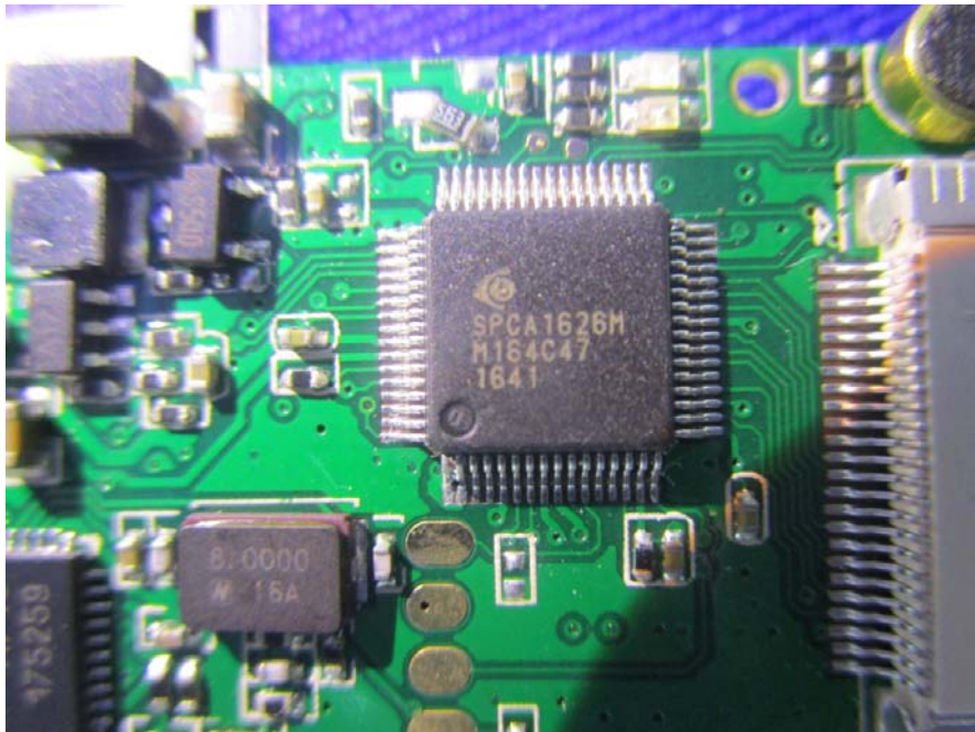
EUT – Camera Mainchip View
