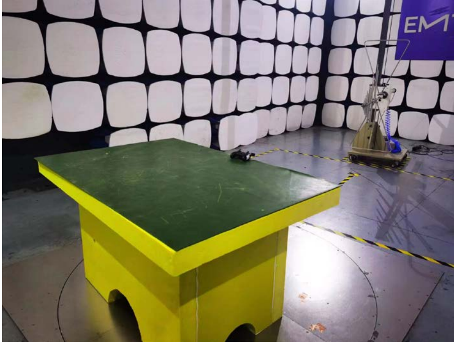
Spurious Emission Test Setup (Above 1GHz)
