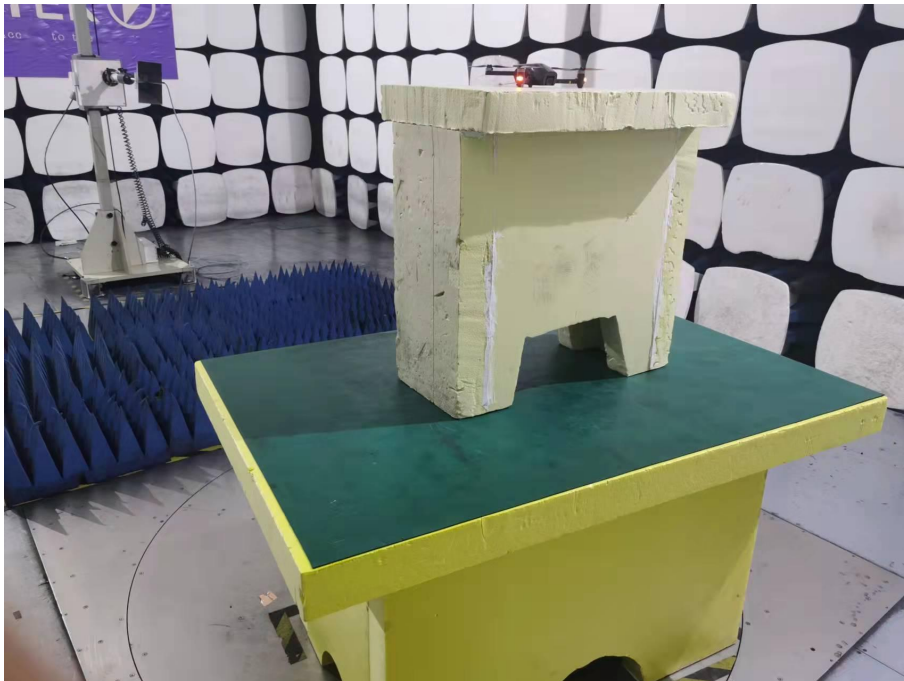
Spurious Emission Test Setup (Above 1GHz)
