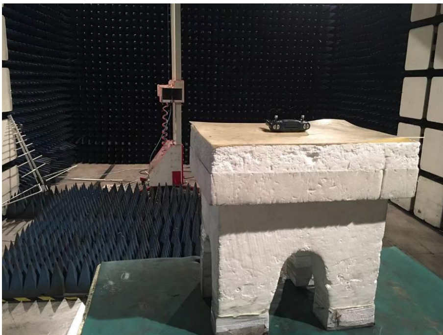
Spurious Emission Test Setup (Above 1GHz)
