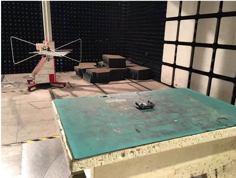
Spurious Emission Test Setup (Below 1GHz)
