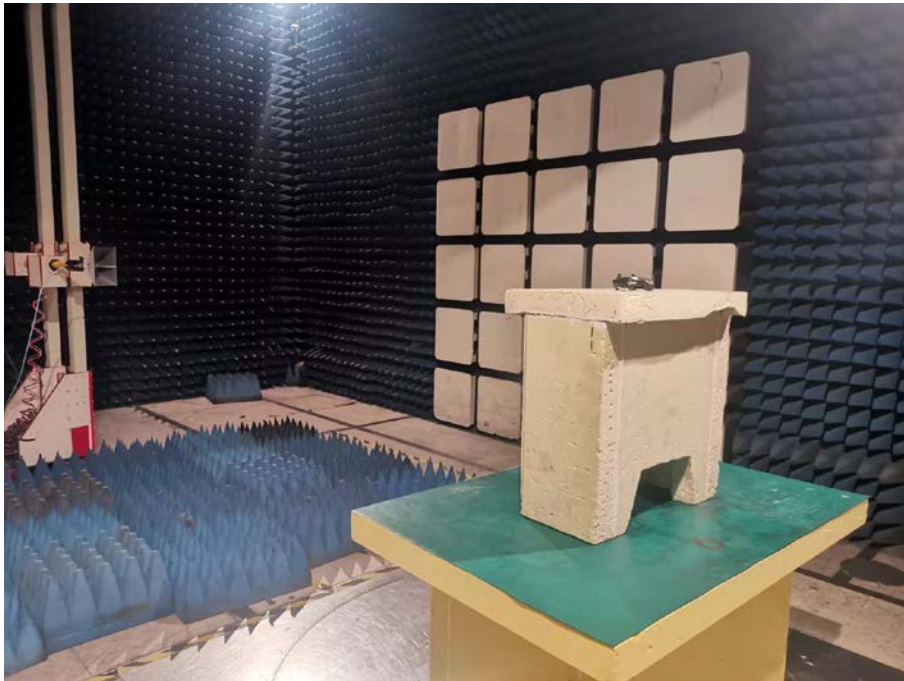
Spurious Emission Test Setup (Above 1GHz)
