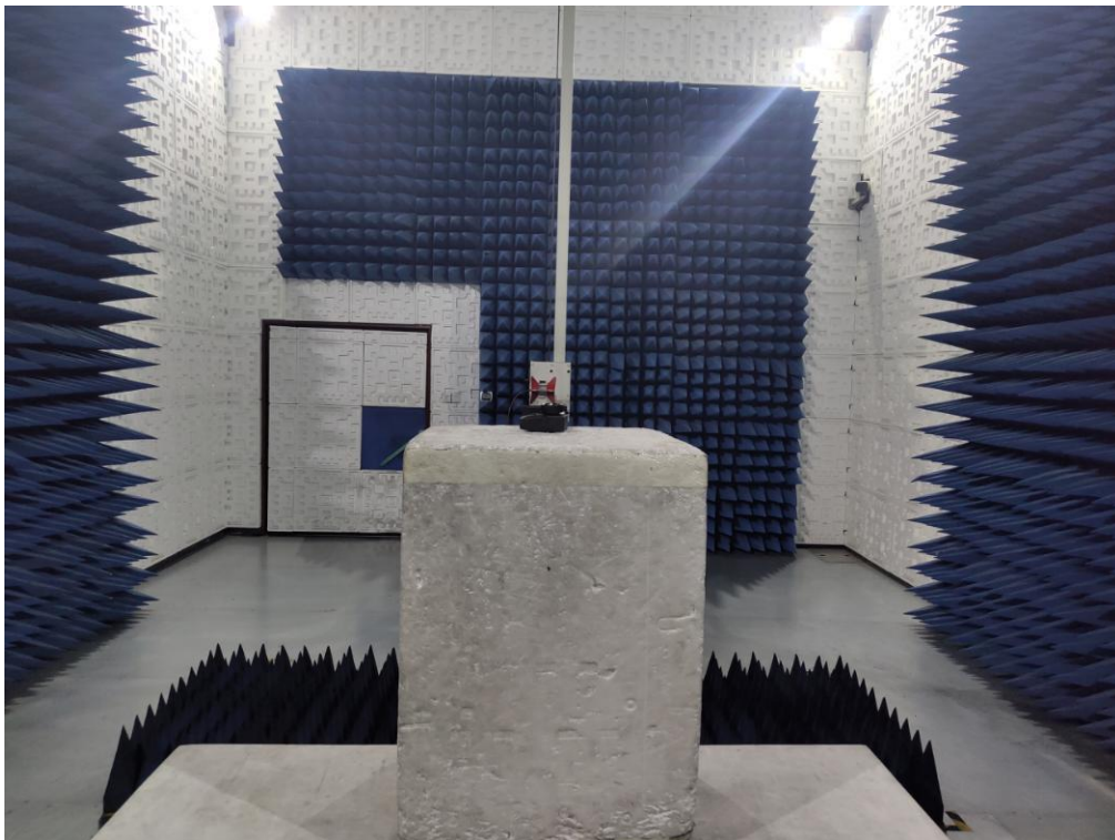
FCC RADIATED EMISSION TEST SETUP ABOVE 1GHZ
