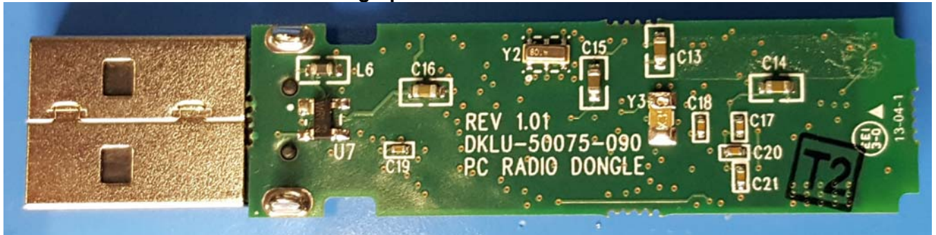
Photograph of PC Board: Foil Side
