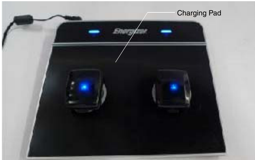
Figure 5. Charging Pad for IMU Battery
