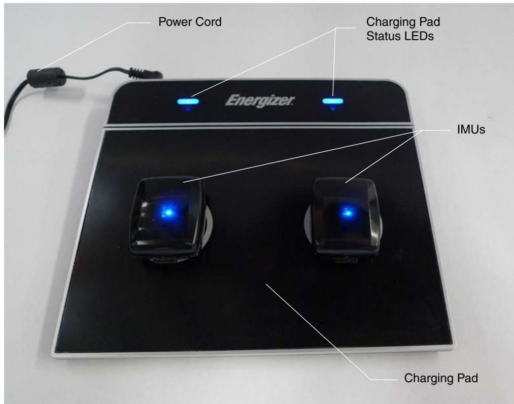
Figure 43. Charging the IMU Battery
