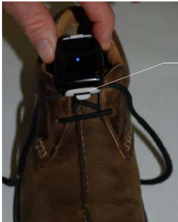
Figure 22. Attaching the Shoe Clip to the Shoe
