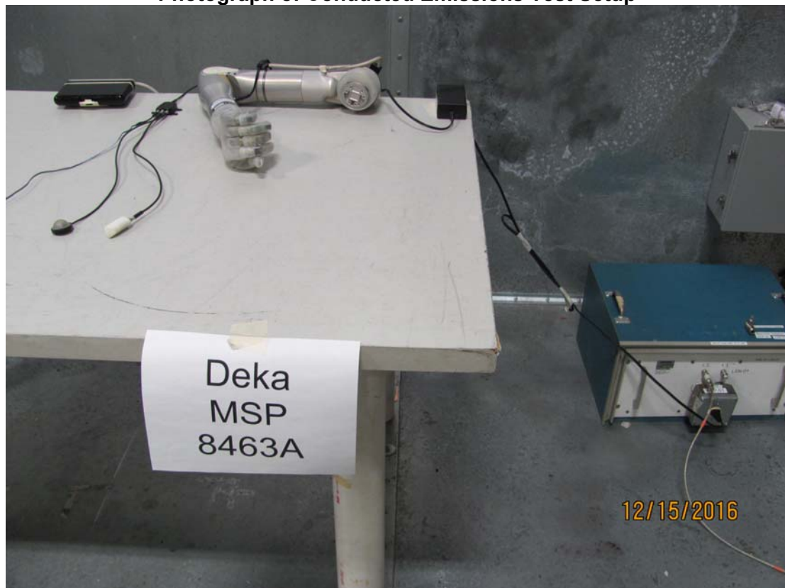
Photograph of Conducted Emissions Test Setup
