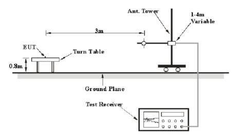
The radiated emission tests were performed in the 3 meters test site, using the setup accordance with the ANSI C63.10-2013. The specification used was the FCC 15.209, and FCC 15.247 limits.
