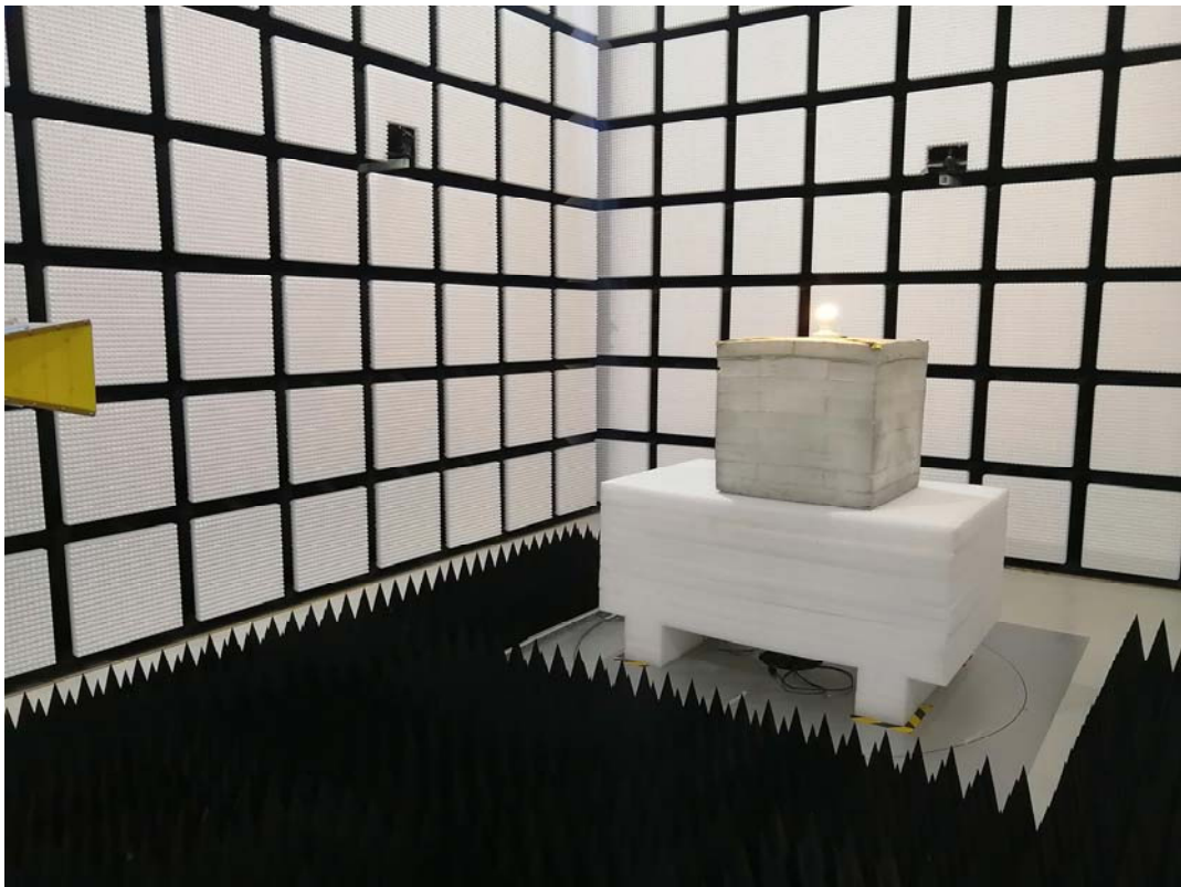
Radiated Emission Above 1GHz View
