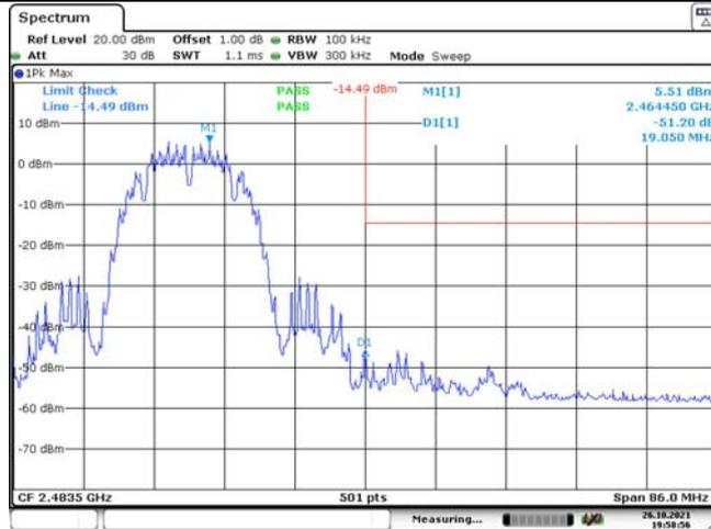
**100 kHz Bandwidth of Frequency Band Edge**
