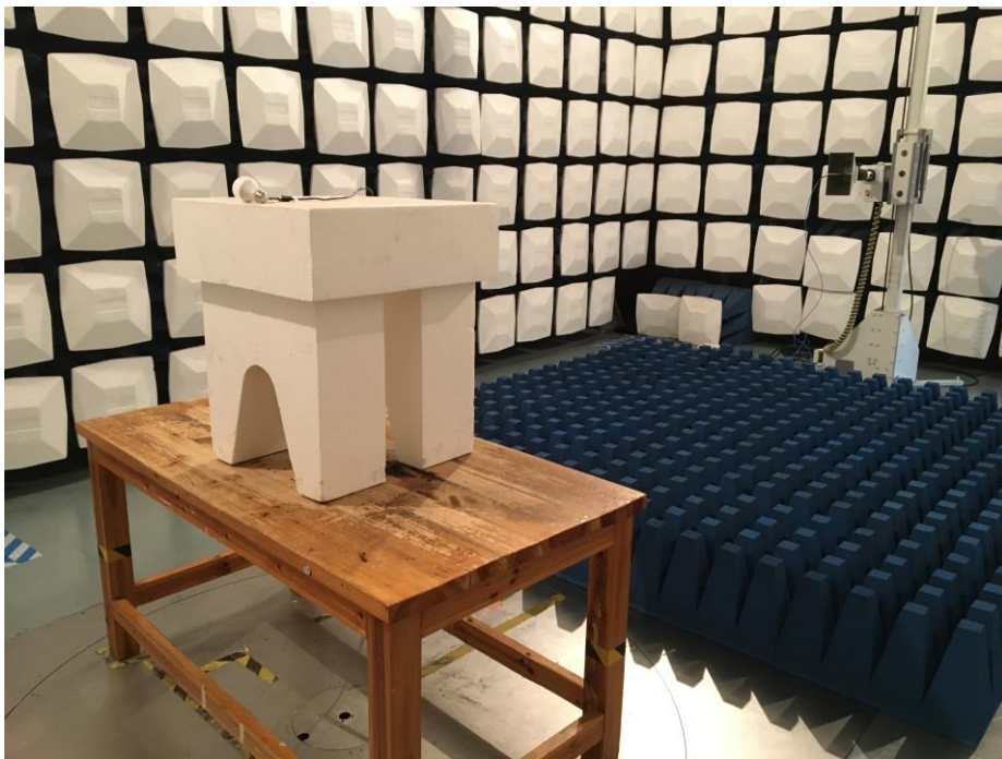
Test Setup For Radiated Emission (Above 1GHz)
