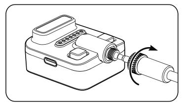
1. Plug in the microphone, and lock it in place by screwing it on clockwise
