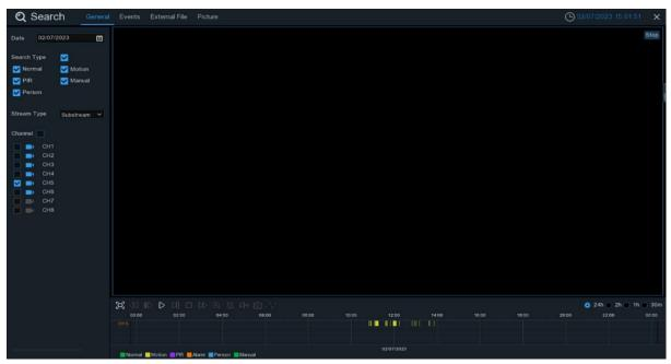
In the playback interface, users can perform operations such as play/stop/single frame playback/clipping/backup, etc. The NVR also supports playback modes such as time slicing, events, and images. Please refer to the user manual for more information. FCC Warning
