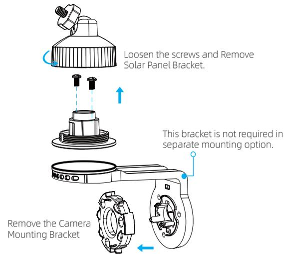
2. Install the mounting bracket of the solar panel in a suitable position.
