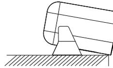
The camera holding bracket can be used for placement and adjustment of angles in some scenarios.
