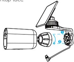
5. Tighten the locking screw on the mount bracket, adjust it to the angle you need, and connect the magnetic extension cord.
