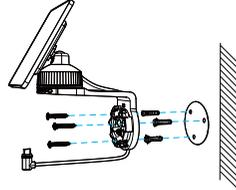
4. Install the camera onto its mounting bracket by turning it clockwise until it clicks into place.
