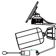
6. Connect the magnetic adapter to the magnetic port of the solar panel.
