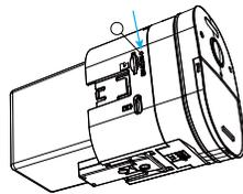
Poke the camera pair button three times within three seconds to start pairing with your NVR. A "Pairing Successful" message should appear on the screen. If you do not see this message, repeat the steps above.
