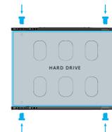
4. Insert and screw the bracket back to NVR, then put the bottom lid back into place.
