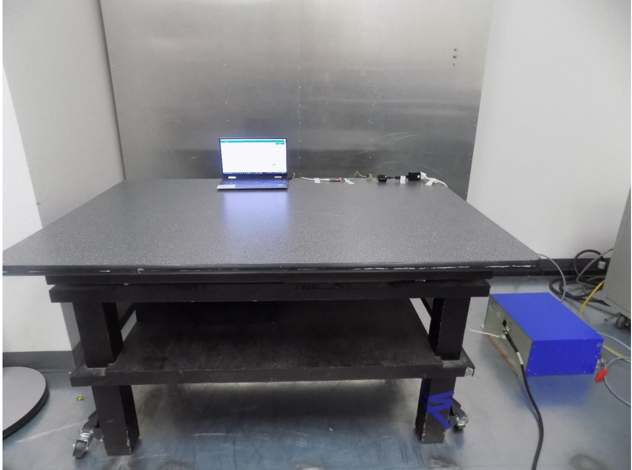
Figure 1: Test Setup for Conducted Emission – Front (EUT battery pack connected to the AC charger)
