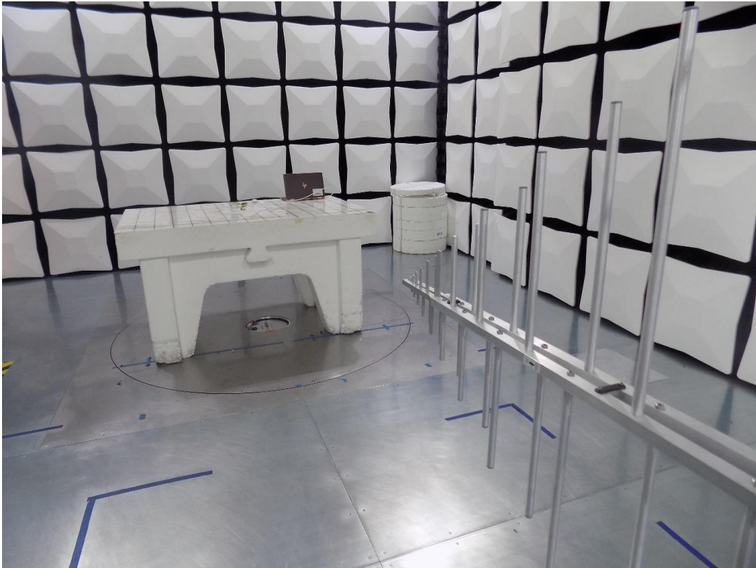
Figure 5: Test Setup for Radiated Emissions 30MHz to 1000MHz - Front View
