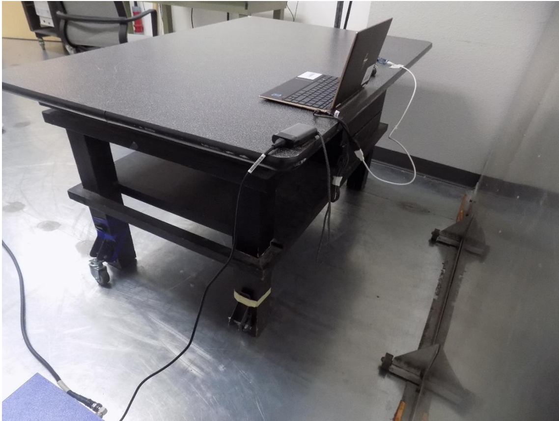
Figure 4: Test Setup for Conducted Emissions – Back (EUT battery pack connected to the Laptop)
