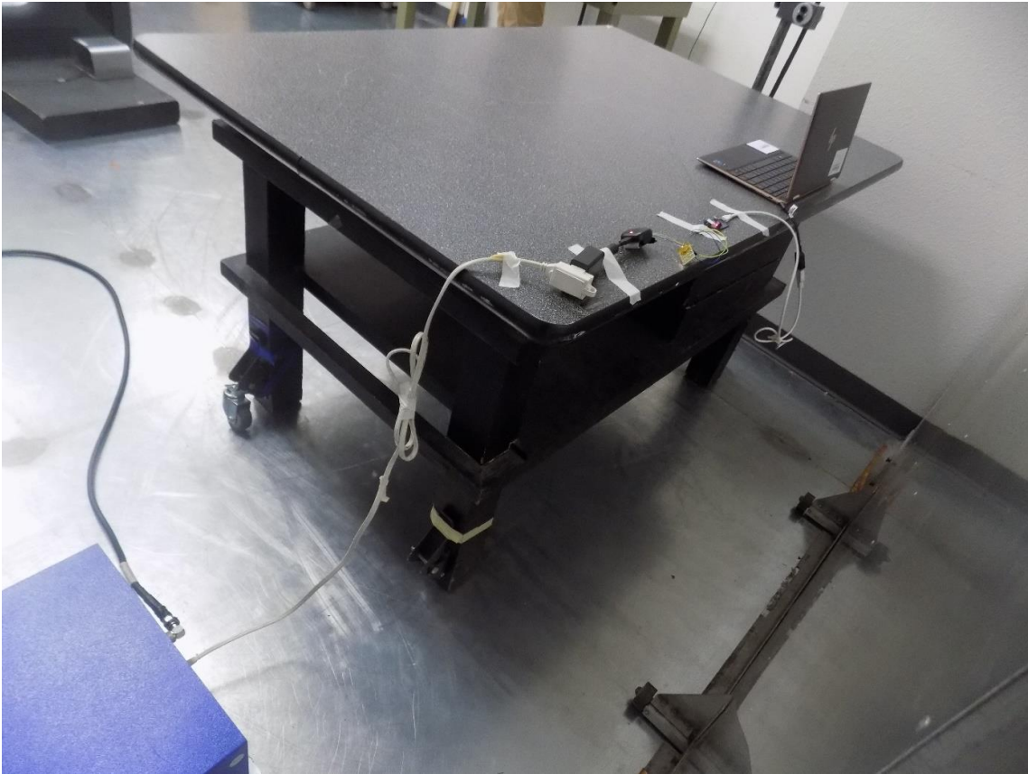
Figure 2: Test Setup for Conducted Emissions – Back (EUT battery pack connected to the AC charger)
