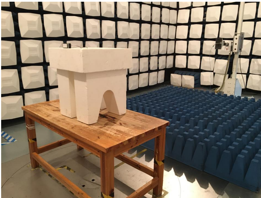
Test Setup For Radiated Emission (Above 1GHz)
