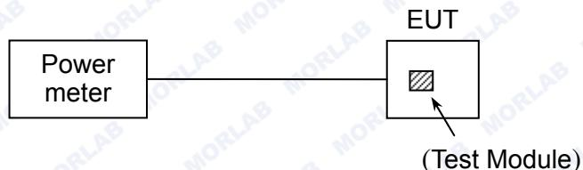
The EUT (Equipment under the test) which is powered by the Battery is coupled to the Power Meter; the RF load attached to the EUT antenna terminal is 50Ohm; the path loss as the factor is calibrated to correct the reading, all test result in power meter.
