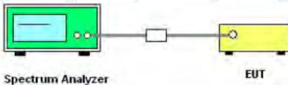
The EUT is coupled to the Spectrum Analyzer; the RF load attached to the EUT antenna terminal is 50Ω; the path loss as the factor is calibrated to correct the reading.
