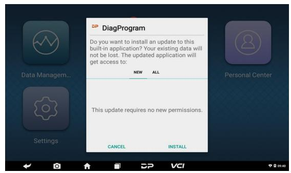
Click "INSTALL" to upgrade and install the APK, after the upgrade and update, a disclaimer will appear and click "Agree" to enter the diagnostic function interface.
