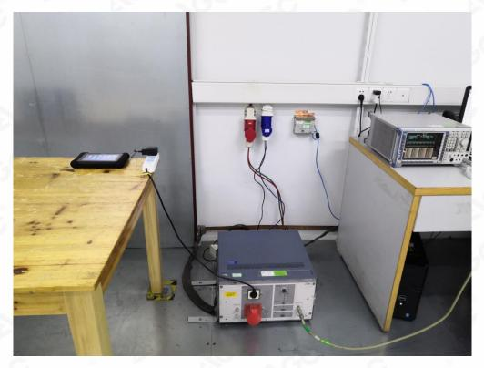
RF CONDUCTED TEST SETUP
