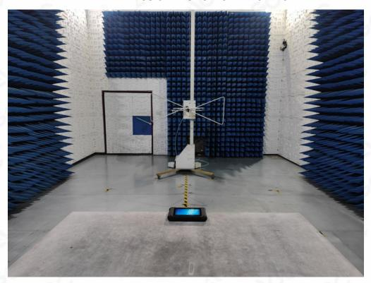
RADIATED EMISSION TEST SETUP ABOVE 1GHz
