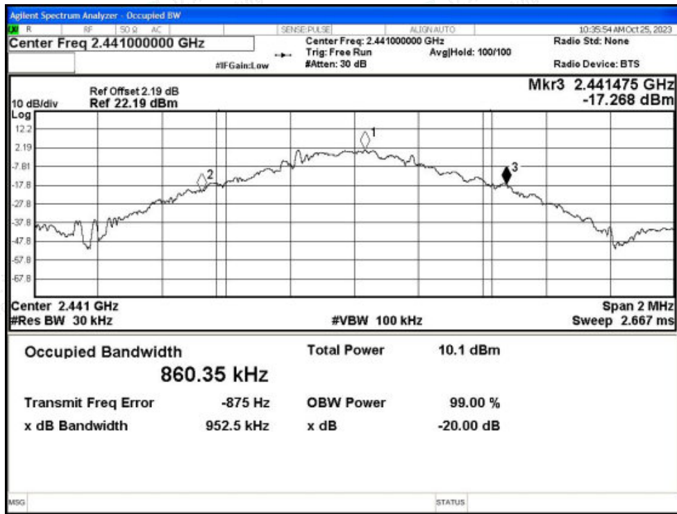
-20dB Bandwidth NVNT 1-DH5 2441MHz Ant1
