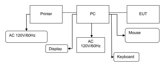
**Equipment Used in Tested System**
